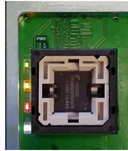
Figure 19: All LEDs flash on startup.
