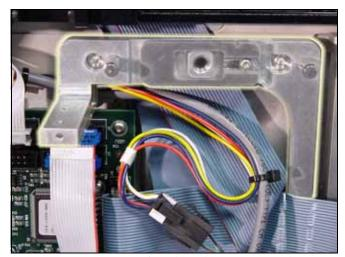
Figure U-6—Adjustable Tape-In Module Base
