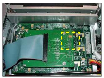
Figure U-45—The Programmer with Ribbon Cable J4 (not shown) disconnected. The NVRAM Battery is on the far side of the next board down.
