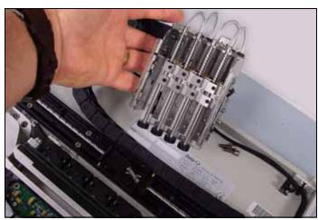
Figure U-37—The PNP Head Partially Removed
