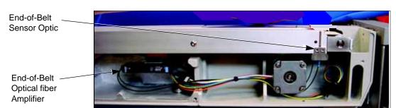
Figure U-25—Reteaching the End-of-Belt Sensor
