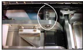
Figure U-9—Some Tape-In Modules have an Adjustable Standoff for setting the Alignment with the Probes. The wrench flats and Locknut identify the Adjustment Stud from a non-adjustable Standoff.
