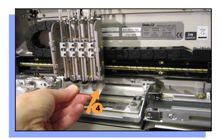
4. When inserting the new precisor, make sure that the part number faces up and that the small holes near the precisor edge fit over the dowel pins on the PNP head.
