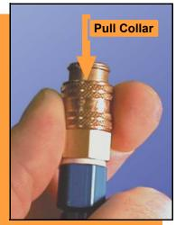
NOTE: The air line is equipped with a "quick connect" that will stop airflow when disconnected.
