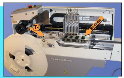
To prevent dust accumulation, inject compressed air into the following component areas:
