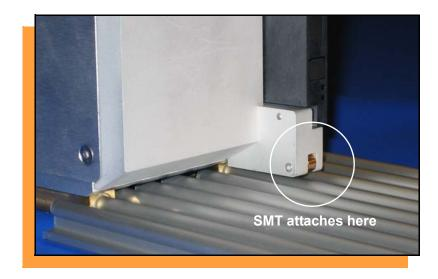
NOTE: The SMT machine should automatically latch onto it.
