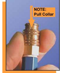
NOTE: The air line is equipped with a "quick connect" that will stop airflow when disconnected.
