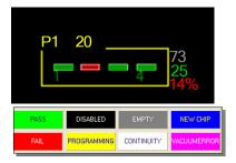
Figure 10: TaskLink's Run window displays socket status by color. This image shows socket two failed programming.
