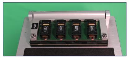
Figure 3: Socket Adapter is installed and bracket tightened..
