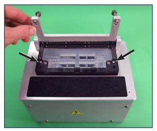
Figure 2: FC Desktop without Socket Adapter.
