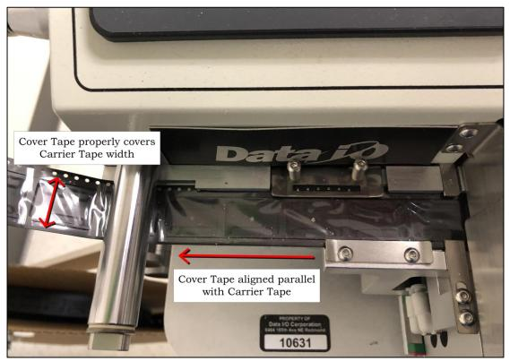
Cover Tape aligned with Carrier Tape
