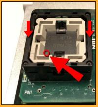
\* For PSV7000, decrease the "Socket Opener Pressure Control" on the main utility panel to approximately 0.25 to 0.3 Megapascals (MPa). Else, excessive socket actuator air pressure can compromise parts longevity.
