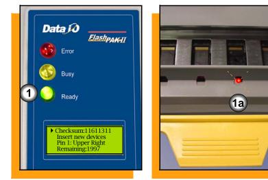
A block of devices is all the devices affected by one push of the actuaor bar (usually four). After each block programming operation the lamps indicate the following:
