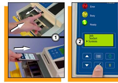
Auto Start is the feature which allows FlashPAK II to begin programming simply by lifting the Actuating Bar (it also closes the sockets). When Auto Start is disabled, you must press Start after closing the sockets to begin programming each block of devices.
