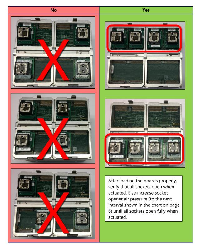
With the UFS Interface Board installed, your LumenX hardware is almost ready for UFS programming. To program a UFS device, you install a device-specific UFS socket adapter on top of the UFS Interface Board (the same as installing a standard LumenX socket adapter).
