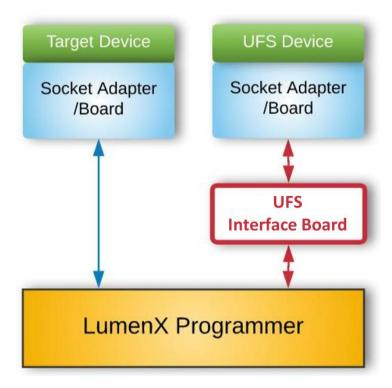
The left side of the diagram above shows a standard LumenX programming job with a socket adapter/board that plugs into the programmer. The right side shows a LumenX programming job for UFS where an additional UFS Interface Board is introduced.
