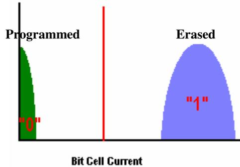
**Figure 1. Cell Current Distribution of an Erased or Programmed Location**
